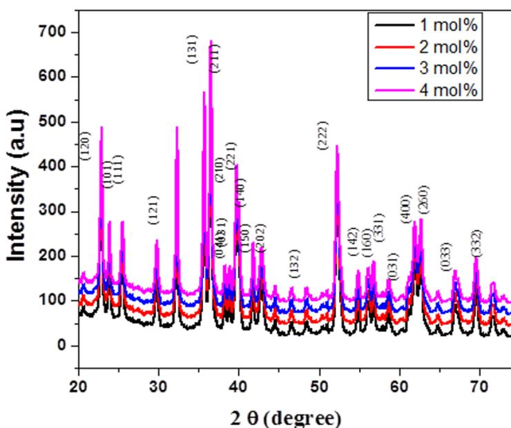
Fig. 1: XRD Pattern of  $\text{Mg}_2\text{SiO}_4:\text{Cr}^{3+}$  (1-4 mol%) nanoparticle
