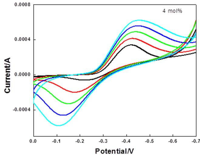
**Fig. 5: CV pattern of  $Mg_2SiO_4:Cr^{3+}$  (4 mol%) nanoparticle**
