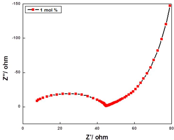
**Fig. 6: EIS pattern of  $Mg_2SiO_4:Cr^{3+}$  (1 mol%) nanoparticle**
