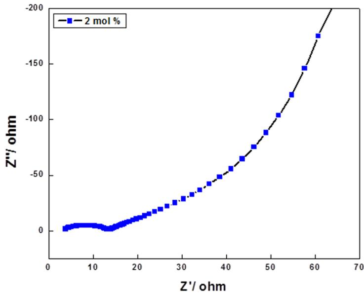
Fig. 7: EIS pattern of  $Mg_2SiO_4:Cr^{3+}$  (2 mol%) nanoparticle
