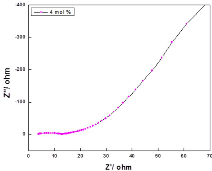
Fig. 8: EIS pattern of  $Mg_2SiO_4:Cr^{3+}$  (4 mol%) nanoparticle
