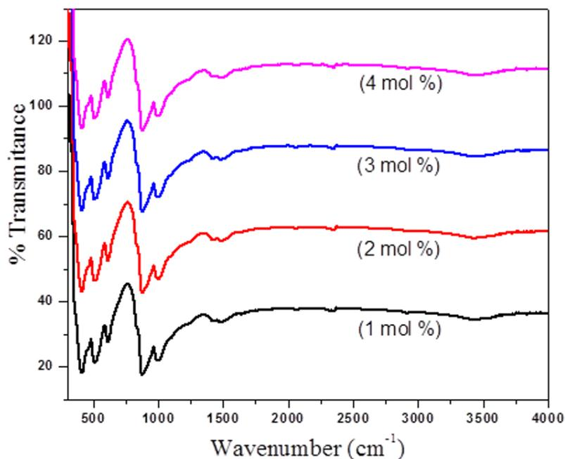
**Fig. 2: FTIR pattern of Mg<sub>2</sub>SiO<sub>4</sub>:Cr<sup>3+</sup> (1-4 mol%) nanoparticle**
