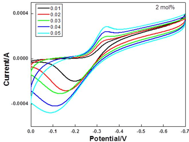
Fig. 4: CV pattern of  $Mg_2SiO_4:Cr^{3+}$  (2 mol%) nanoparticle
