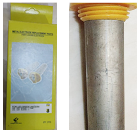
Fig.4: Magnesium alloy electrodes used in this study
