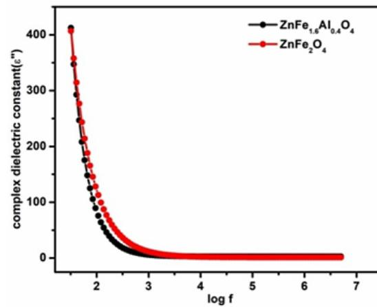
Fig. 4b: Complex dielectric constant of  $\text{ZnFe}_{2-x}\text{Al}_x\text{O}_4$  ( $x=0.0$  &  $0.4$ ) with frequency
