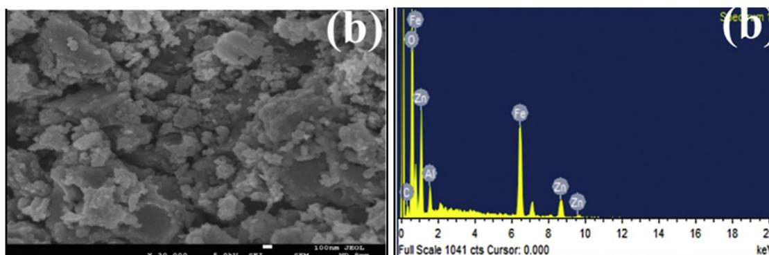
**Fig. 3 (b): SEM micrographs and EDX analysis of  $ZnFe_{1.7}Al_{0.3}O_4$** **Table 2 (b): Elemental analysis of  $ZnFe_{1.7}Al_{0.3}O_4$**
