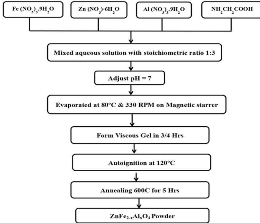
Fig.1: Flowchart of synthesis process preparing ZnFe<sub>2-x</sub>Al<sub>x</sub>O<sub>4</sub> sol gel autocombustion method
