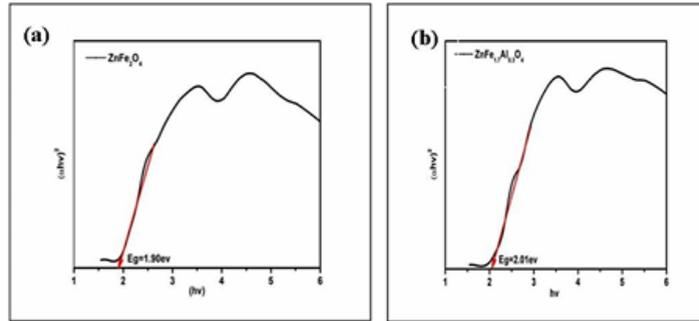
Fig. 4. (a, b): UV-Vis plot of plot of nanoparticles  $ZnFe_{2-x}Al_xO_4$  ( $x=0.0, 0.3$ )
