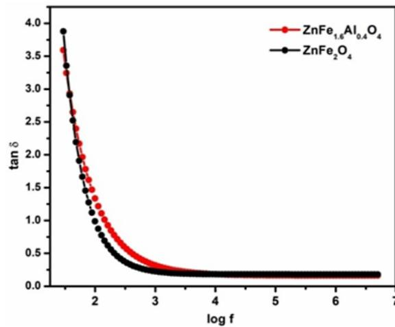
Fig. 4c: Loss tangent of  $\text{ZnFe}_{2-x}\text{Al}_x\text{O}_4$  ( $x=0.0$  &  $0.4$ ) with frequency
