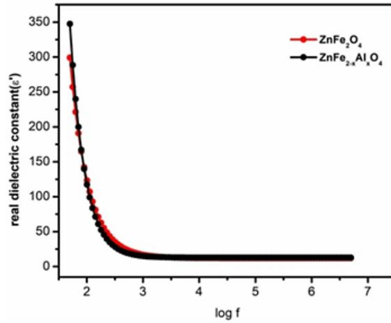
Fig. 4a: Real dielectric constant of  $\text{ZnFe}_{2-x}\text{Al}_x\text{O}_4$  ( $x=0.0$  &  $0.4$ ) with frequency
