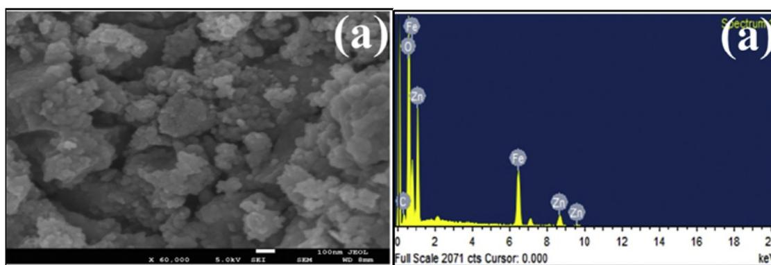
**Fig. 3 (a): SEM micrographs and EDX analysis of  $\text{ZnFe}_2\text{O}_4$**
