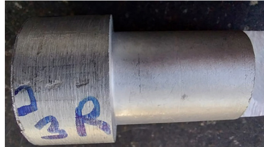
Fig. 4: (a) Macro photograph of Machined Specimen P3R1-Ra=1.514 μ
