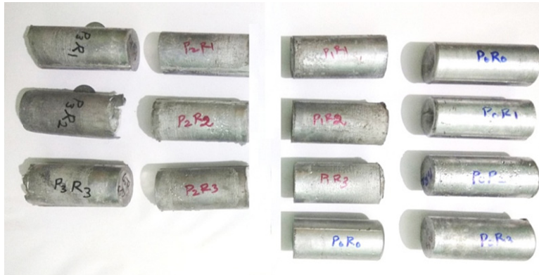
Fig.1: Specimens made by altering the weight percentage of reinforcement & squeeze pressure
