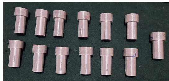
Fig. 3: Squeeze cast specimens after turning operations
