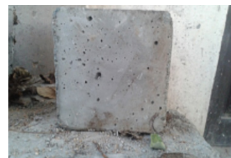
Fig. 9: Concrete Cube after Durability Test
