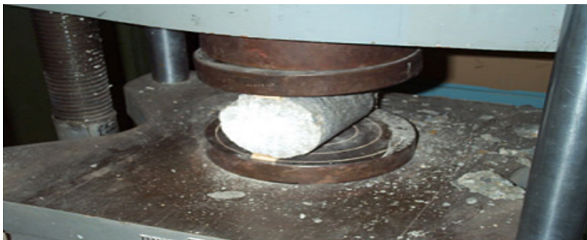
Fig. 6: Specimen under Split Tensile Strength Test
