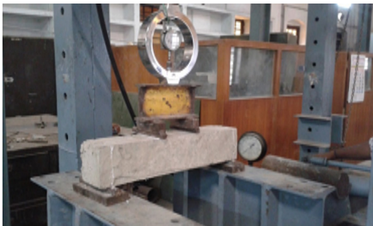
Fig. 7: Specimen under Flexural Strength Test
