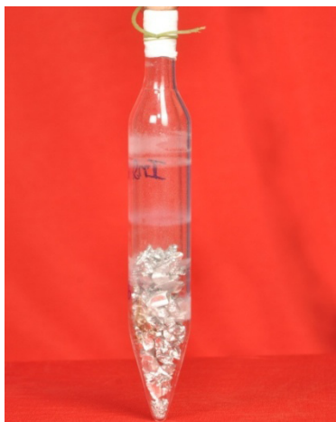
Fig. 3: Vacuum sealed crucible containing Ga, Sb raw materials
