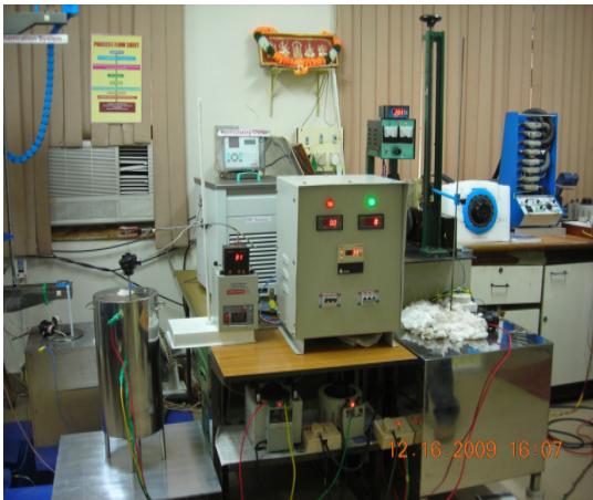
Fig.1: Directional freezing system
