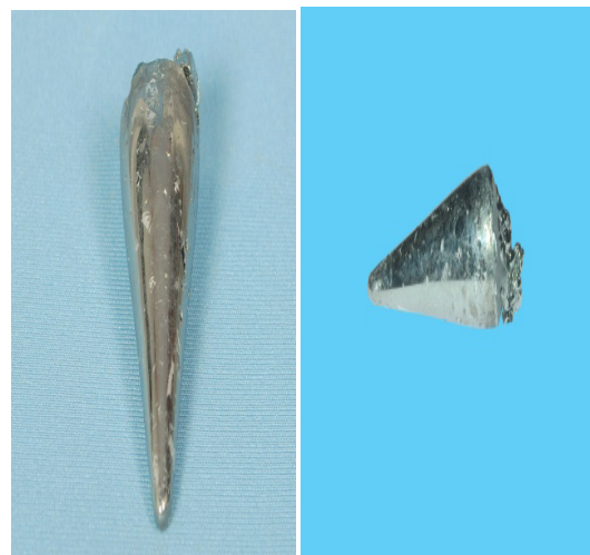
Fig. 4: Purified and crystallised GaSb
