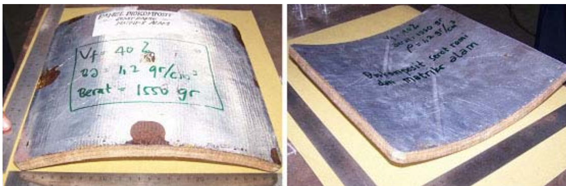
Fig. 13: Sample of curve panel from ramie fibers reinforced matlac matrix biocomposite
