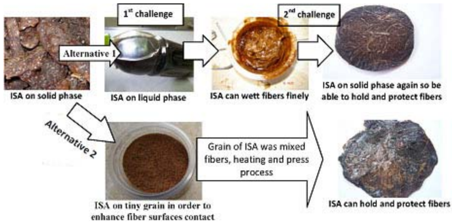
Fig. 5: Two methods that can be identified to engineer ISA become matrix composite
