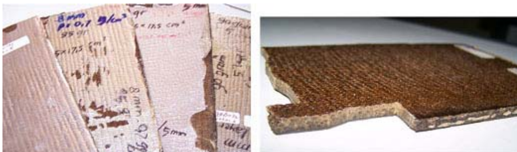
Fig. 12: Sample of ramie fibers reinforced matlac matrix biocomposite
