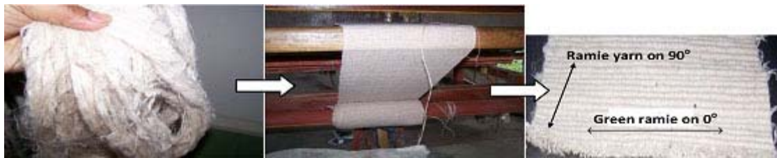
(a) ramiee fiber (b) ramiee fiber weave process (c) plain weave of ramiee fiber
