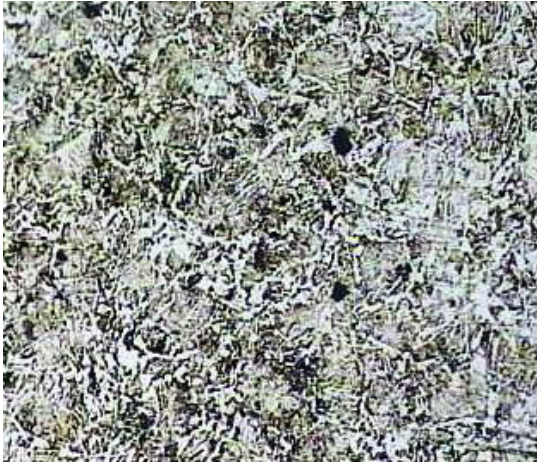
Fig. 10: Microstructure of weld metal for, I=110A, S=62cm/min and V=25v 1000 ×
