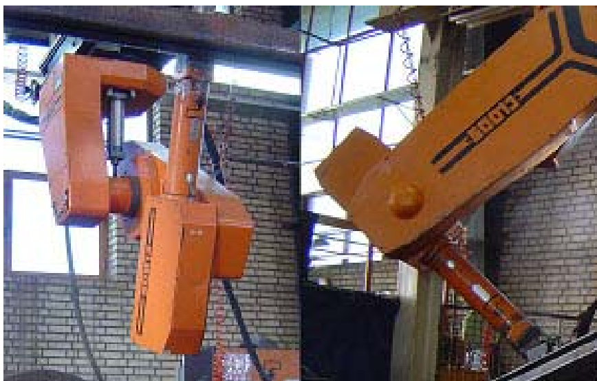
Fig. 1: The CO 2 arc welding robot and its apparatus used in experiments
