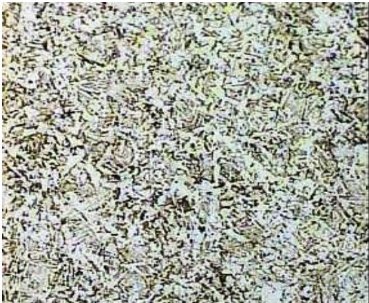
Fig. 6: Microstructure of weld metal for V=25v, S=62cm/min and I=100A 1000x
