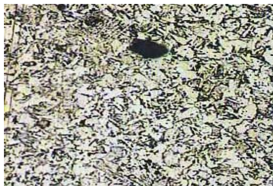
Fig. 14: Microstructure of weld metal for V=25v, I=110A and S=82cm/min 1000×
