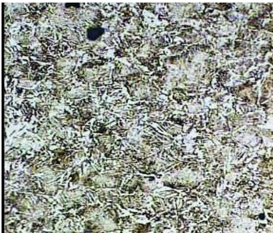
Fig. 12: Microstructure of weld metal for V=25v, I=110A and S=42cm/min 1000×
