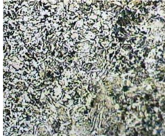
Fig. 7: Microstructure of weld metal for V=25v, S=62cm/min and I=110A 1000x
