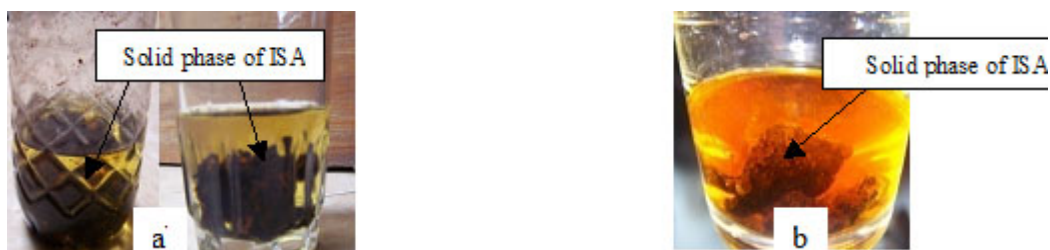
Fig. 8: ISA did not dissolve in non polar solvent (a) ISA remained in solid phase due to its no solubility in gasoline and kerosene (b) ISA remained in solid phase due to its no solubility in acetone
