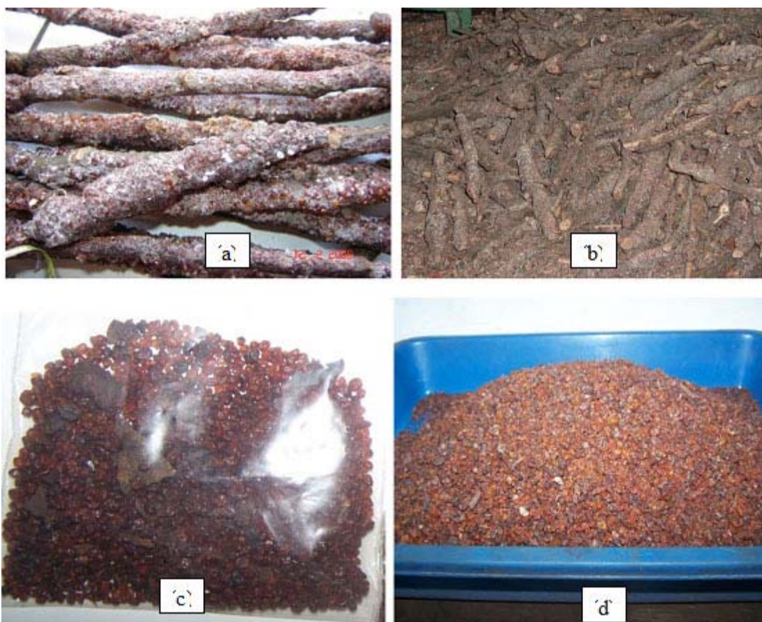
Fig. 11: (a) Lac insect secretion on Albazia tree (b) Lac insect secretion at Kesambi tree (c) Lac insect secretion on Albazia tree which was granulated to pass mesh 10 (d) Lac insect secretion on Kesambi tree which was granulated to pass mesh 10
