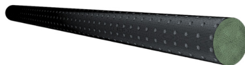
Fig. 2: Meshing of simple pipe with dimple
