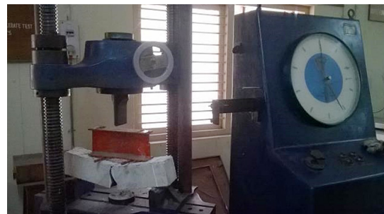
Fig. 8: Flexural Testing of Beam Specimen
