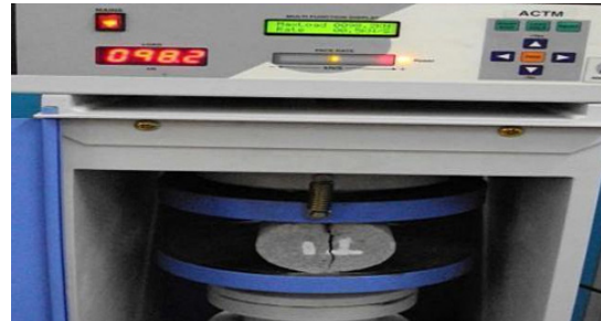
Fig 9: Splitting Tensile Strength test under progress (self made)
