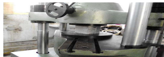
Fig 7: Cube compressive strength test under progress(self made)
