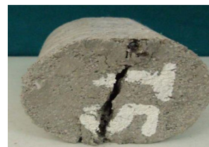
Fig 16: Failure due to Split tensile (self made)
